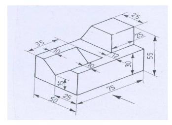
**8.** Draw three views of the blocks shown pictorially in figure according to [10M] first angle projection
